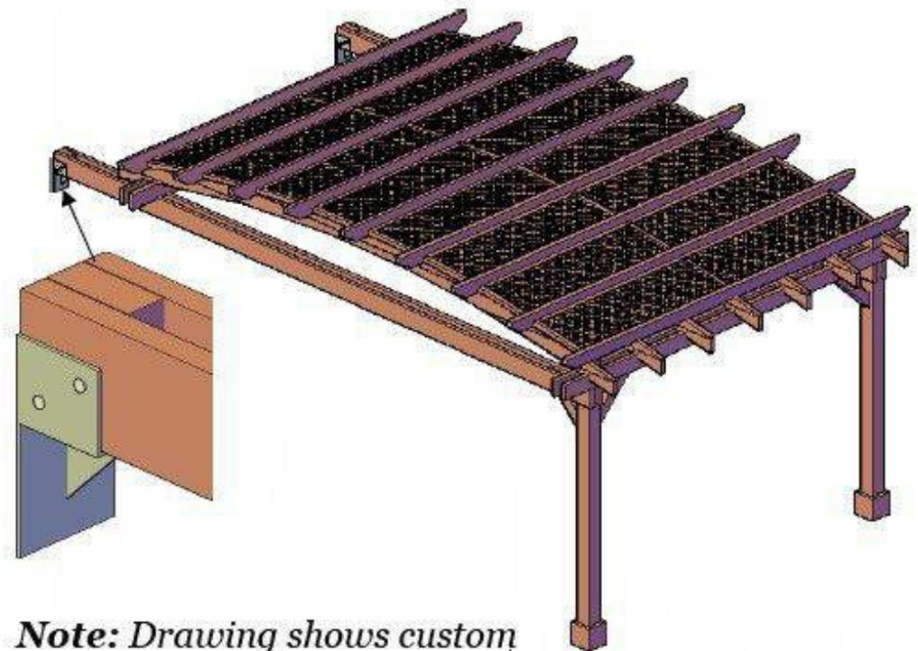
**Note:** Drawing shows custom steel anchors and extra supports to clear a low eave.
